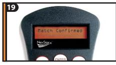
Repeat the process for the third alignment star. When the telescope has been aligned to the final star, the display will read "Match Confirmed". Press UNDO to display the names of the three bright objects you aligned to, or press ENTER to accept these three objects for alignment.
